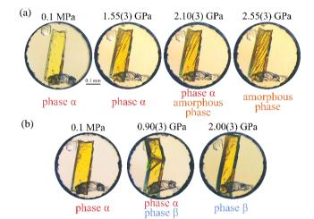
Figure 1. The sample C5-PPB single crystal (a) first compressed rapidly to 1.5 GPa, when the wrinkles mark the onset of amorphization, and then (b) after releasing pressure it was compressed again slowly to 0.9 GPa, where the transition to phase  $\beta$  starts and transition fronts travel through the sample, till it all transforms to the end.
