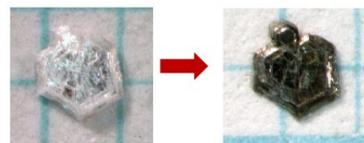
Fig.3 Optical view of hBN and wBN crystals.
