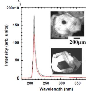
Fig.2 CL spectra of hBN crystals. Inset: 215nm CL image
