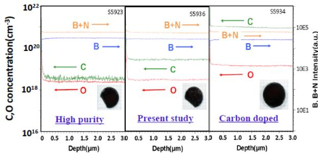
Fig.5 SIMS depth profiles of cBN sintered bodies with different Carbon content.
