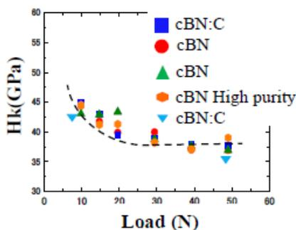
Fig.6 Knoop hardness of binderless cBN sintered bodies with different carbon content.
