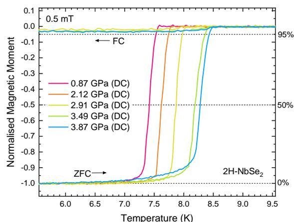
Figure 1.  $M(T)$  sweeps for 2H-NbSe<sub>2</sub> in the Magnetic Property Measurement System (MPMS) compatible gemstone anvil cell.
