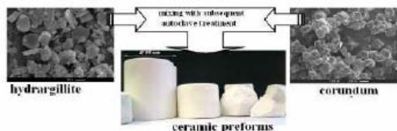
Fig.1 Scheme of preparation of ceramic preforms
