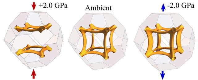
Figure 1. Constant-energy surfaces in the Brillouin zone of PbTe under uniaxial stress. The change in topology observed for compressive stress indicates changes to band extrema near the Fermi level, which play a crucial role for thermoelectricity.
